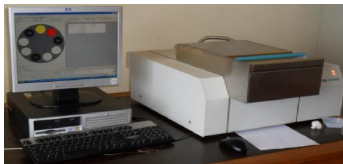
Fig. 4 The picture of the Spectro Xepos™ spectrometer
