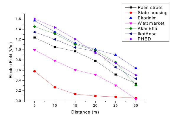
**Figure 1**: Variation of electric field with distance at various sample locations
