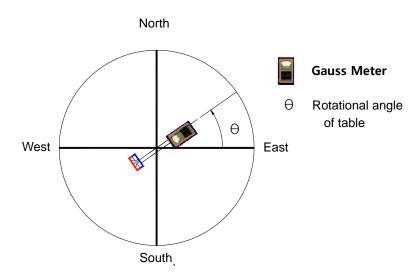
Fig. 2. In the first experiment, the permanent magnet and the magnetic sensor are fastened to the rotational table which is set to be parallel to the horizontal plane.
