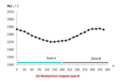
Fig. 6. Net magnetic flux density during 360 degree of vertical rotation of the table for type-A and Type-B
