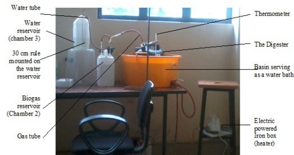
Fig-9 The setup of the laboratory scale biogas digester system
