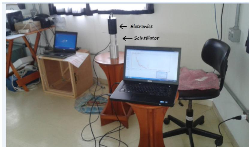
**Figure-1.** View of the gamma scintillator with associated electronics and computer.
