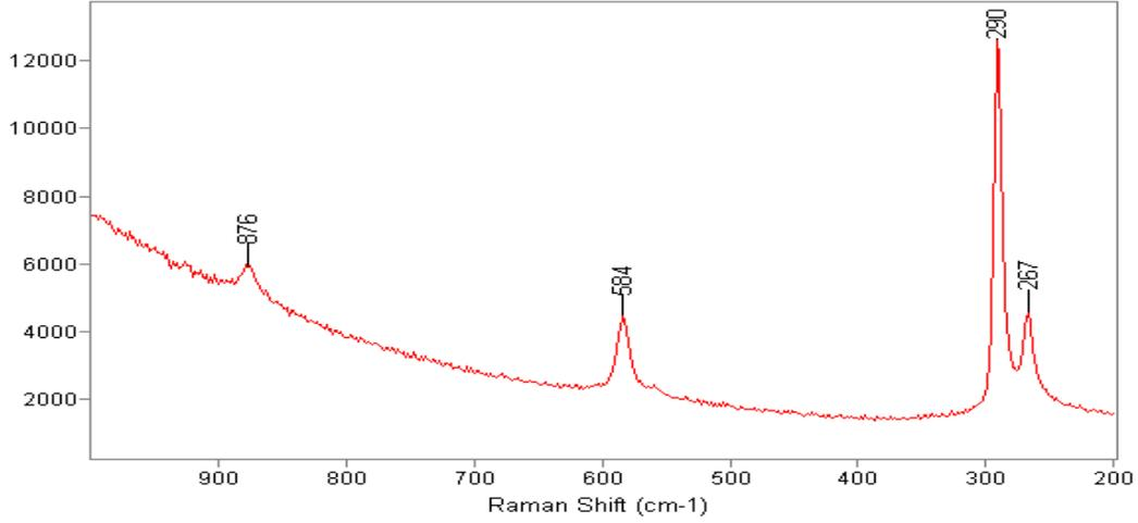
**Fig. 1(b). Raman scattering spectrum for  $\text{Al}_{0.28}\text{Ga}_{0.72}\text{As}$  super-lattice at room temperature**
