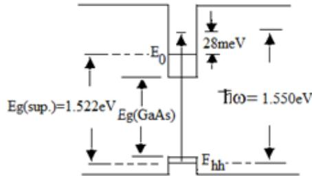
**Fig. 3. Schematic representation of multi-phonon Raman scattering for GaAs/Al<sub>0.28</sub>Ga<sub>0.72</sub>As super-lattice**
