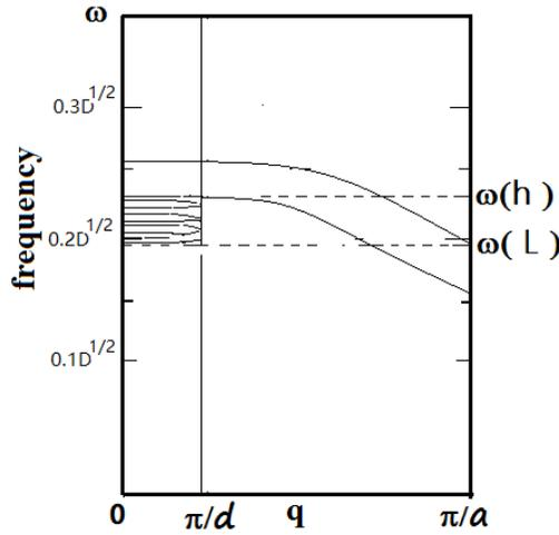
**Fig.2. The dispersion relations of optical phonons of linear chain of GaAs (a) and of  $\text{Al}_{0.28}\text{Ga}_{0.72}\text{As}$  (b) , and optical phonon folding for GaAs/  $\text{Al}_{0.28}\text{Ga}_{0.72}\text{As}$**
