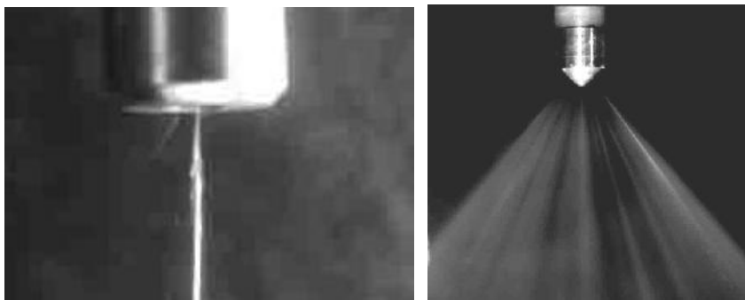
Fig. 2: Photographs of the ejecting aerosoles from the nozzle of high pressure injector under two different conditions.
