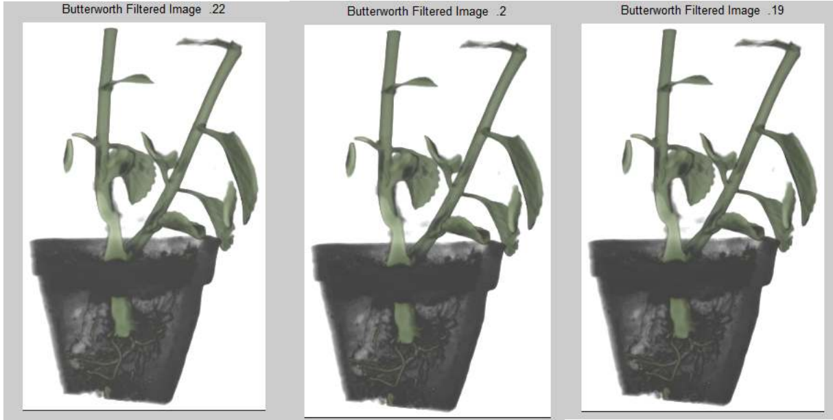
Fig. 9. Processed image by modified Butterworth low-pass filter with different f_c values.
