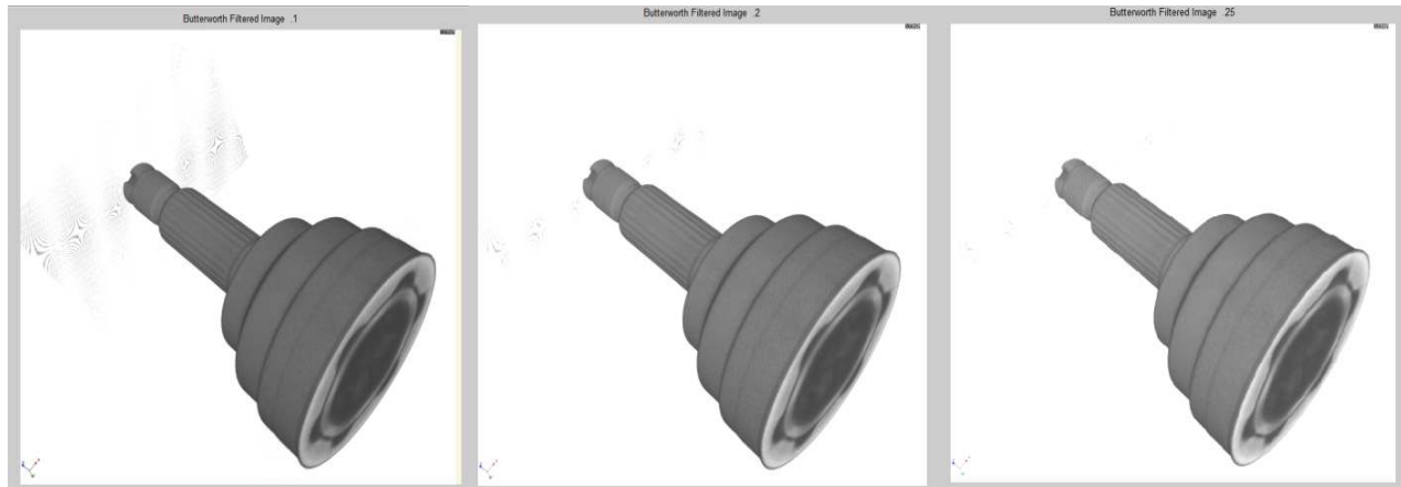
Fig. 10. Processed image by modified Butterworth low-pass filter with different f_c values.
