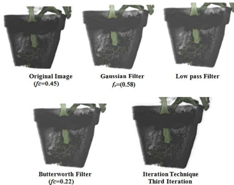
Fig. 14. Enhancement techniques in the root part of the plant. The iteration module is potentially effective.
