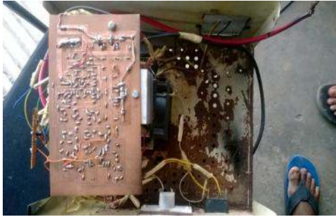
Fig 19: packaging of the UPSz into a casing.
