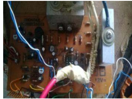
Fig 20: picture of the motherboard of the UPSz
