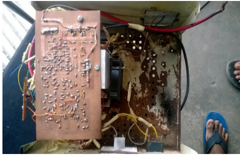
Fig 19: packaging of the UPSz into a casing.
