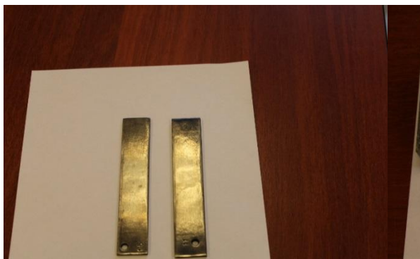
Fig.2c Steel samples Experiment No. 1 (sample 11, right) the wanted signal is 6 dB, the transverse fissure of the doped layer, the depth of the 2 micron..The steel sample .Experiment No. 2 (15 a sample left) transverse fracture of alloyed layer, the useful signal is 12 dB depth of 9.5 microns.
