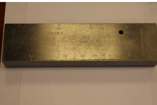
Fig.2.d Steel bar (standard sample) experiment No. 4 size 210x59x30 mm Steel 20 delay 20 MS at a length of 59 mm. the Useful signal 2-4 dB.
