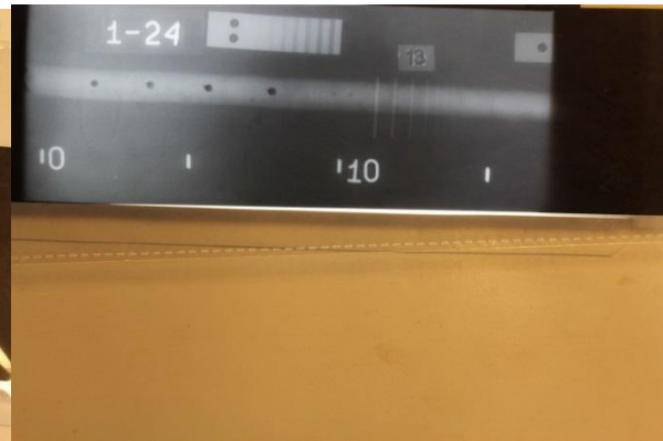
Fig.1b x-ray the weld in the experiment No. 3, the desired signal 12 dB the picture shows 4 empty holes
