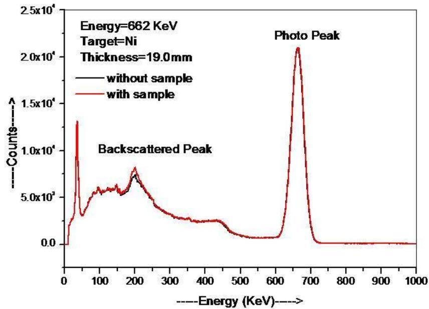
Figure 2: The backscattered peak (200.91 keV) and photo peak (662 keV) with Nickel sample (thickness 19.0 mm) using  $^{137}\text{Cs}$  radioactive isotope
