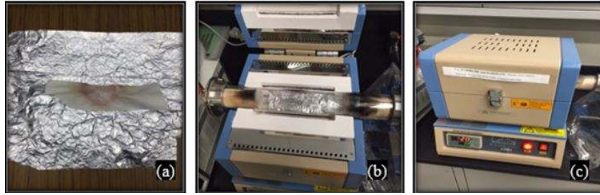
Fig. 3 Photos showing (a) Sample ready to be wrapped in aluminum foil prior to heat treatment, (b) Sample placed in a MTI tube in the furnace prior to heat treatment, (c) Heat treatment of the sample in the furnace at 500°C.
