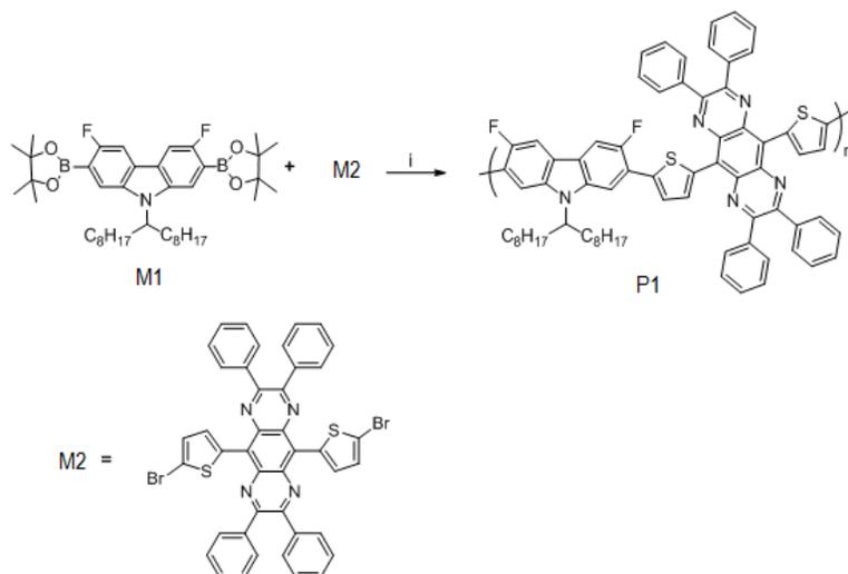
**Scheme1: Preparation of polymer P1 (i) Pd(AcO)<sub>2</sub>, tri-*o*-tolylphosphine, NaHCO<sub>3</sub>, THF**
