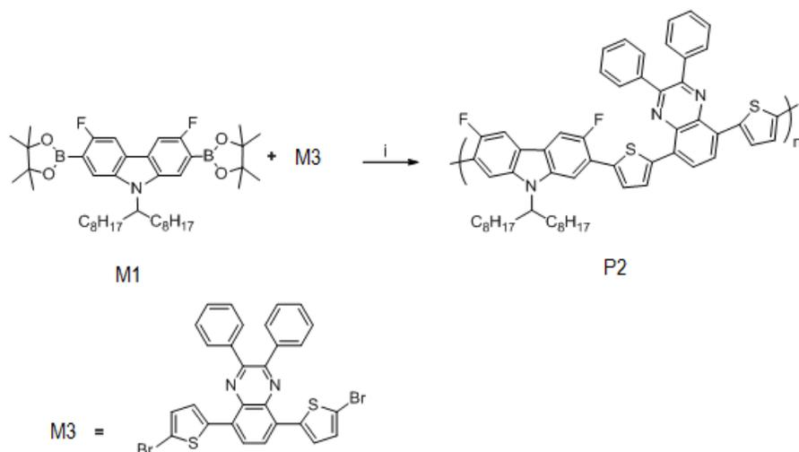
**Scheme2: Preparation of polymer P2 (i) Pd(AcO)<sub>2</sub>, tri-*o*-tolylphosphine, NaHCO<sub>3</sub>, THF**
