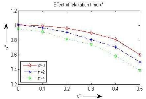
**Fig. 2.** The growth rate of instability is plotted against the dimensionless wave number  $k^*$  with variation in the relaxation time  $\tau^* = 0, 2, 4$ , with taking the values of  $k_s^*, \nu^*, k_1^*$  and  $\lambda^*$  as unity.
