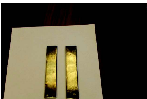
Fig.2c Steel samples Experiment No. 1 (sample 11, right) the wanted signal is 6 dB, the transverse fissure of the doped layer, the depth of the 2 micron..
