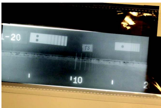
Fig.1A x-ray of the weld of experiment No. 6, the wanted signal is 14 dB. In the picture under the welding cracks.
