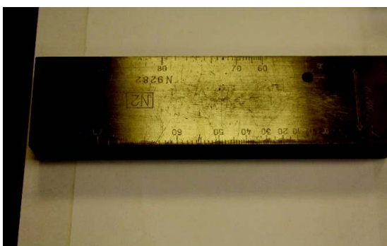
Fig.2.d Steel bar (standard sample) experiment No. 4 size 210x59x30 mm Steel 20 delay 20 MS at a length of 59 mm. the Useful signal 2-4 dB.
