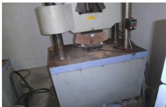
114 Figure 1: Test of resistance in inflexion (three points) on CEB
