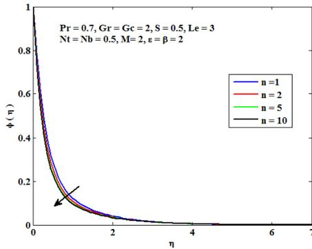
Fig11: Concentration profile with variation in Non linear stretching parameter n
