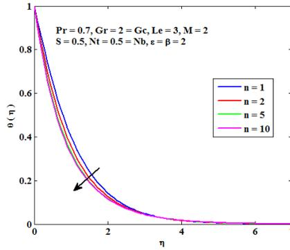
Fig 12: Temperature profile with variation in nonlinear stretching parameter n
