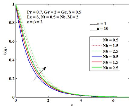
Fig 8: Temperature profile with variation in Brownian motion parameter
