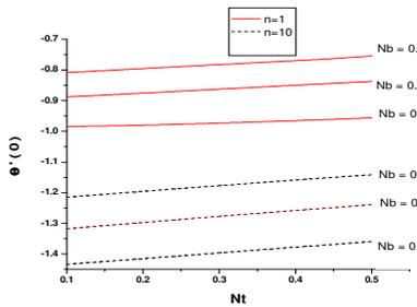
Fig 13: Variation of local Nusselt number  $-\theta'(0)$  with Nt for different values of Nb.
