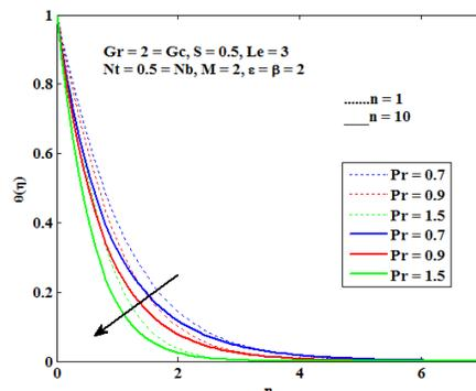
Fig 10: Temperature profile with variation in Pr
