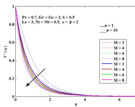
Fig 2 : Velocity profile with variation in M
