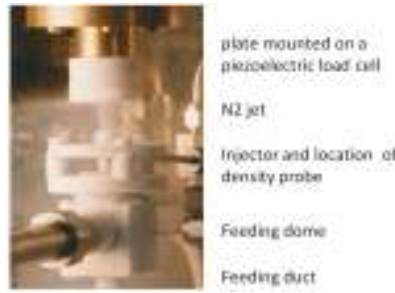
105 106 Fig. 3. LN2 two-phase jet exiting the injector (vertical flow) and impacting the plate 107 mounted on load cell: the N2 flow goes upwards on the picture
