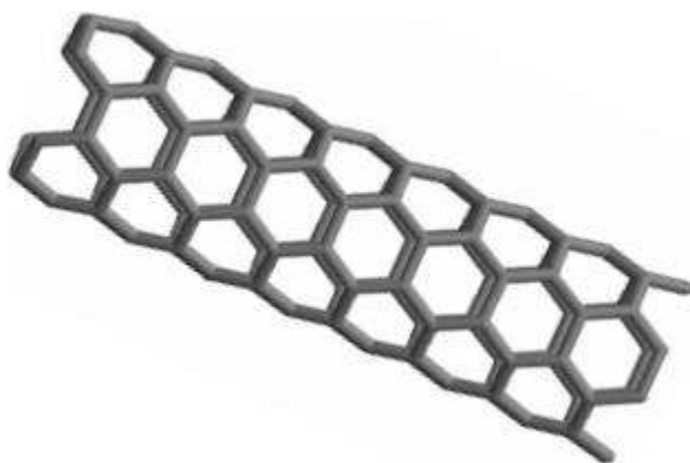
54 55 Fig. 1. The 3-Dimensional Lattice of Armchair Polyhex Nanotubes TUAC_6[m,n] 56 (\forall m, n \in \mathbb{N}) .
