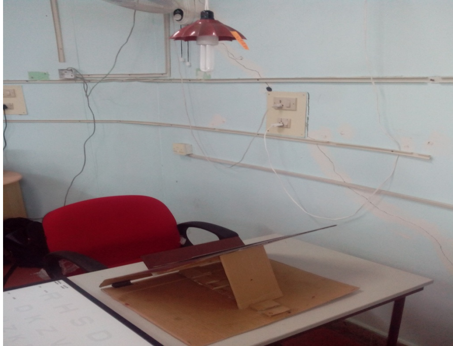
Figure-1 Experimental seating arrangement of participant for reading ischihara colour vision plates under different lighting sources.
