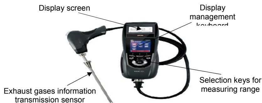
Fig. 1. Device used for measurement of exhaust gases from motorcycles
