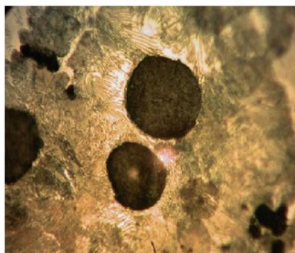
Figure 1: Micrograph of as-cast ductile iron showing graphite nodules in a pearlitic matrix with free carbide (light irregular particles), 2% nital etched x 500.
