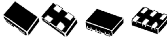
Fig. 2. Typical molded COL package outline
