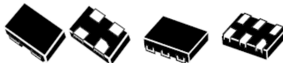
Fig. 2. Typical molded package outline
