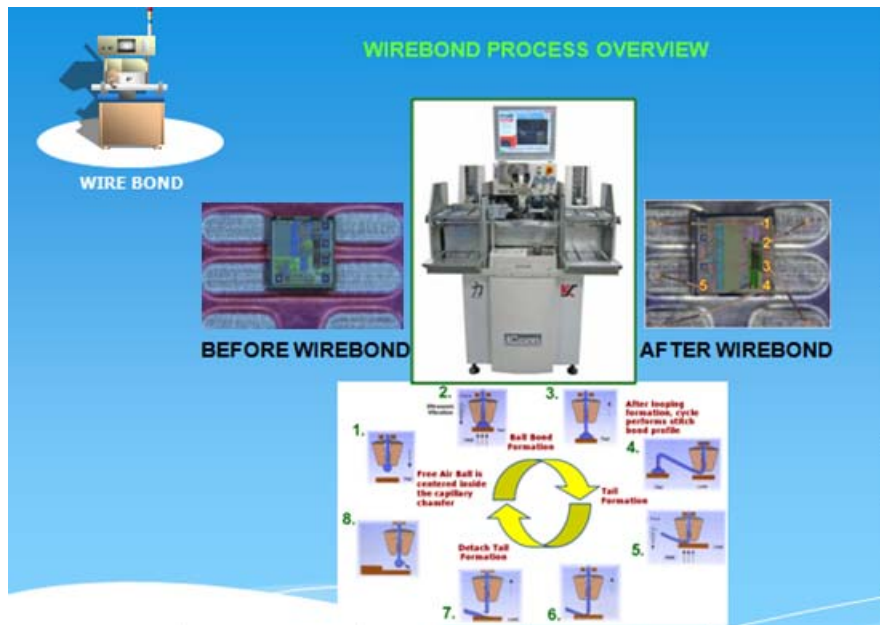
87 88 89 Fig. 3. Wirebonding process mechanism 90
