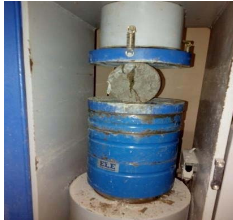
Fig. 3. Split-Tensile testing of concrete cylinder
