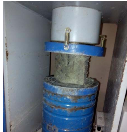
Fig. 1. Compressive strength test of concrete cube
