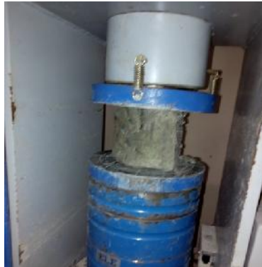
Fig. 1. Compressive strength test of concrete cube
