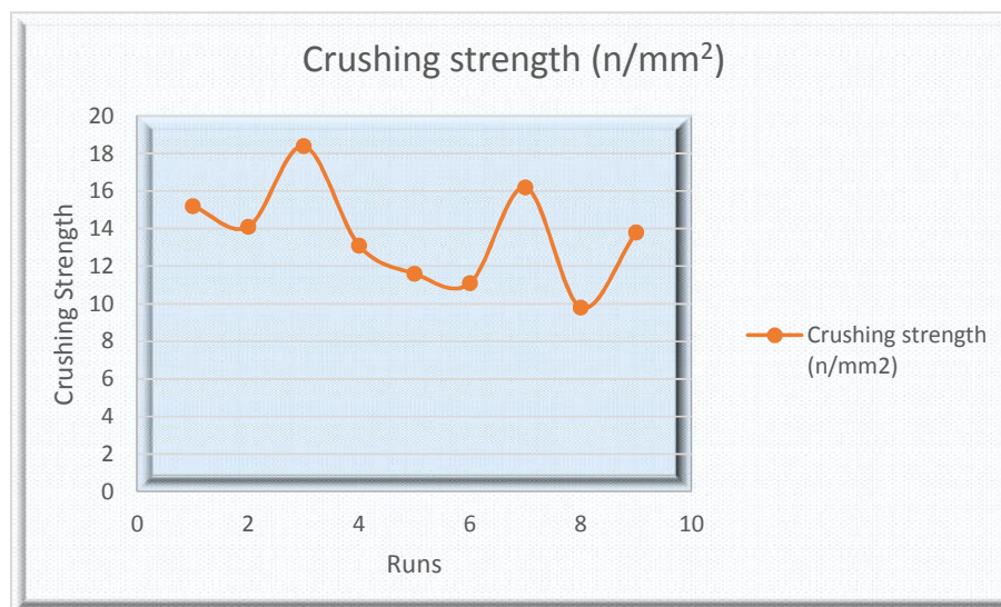
Fig 4: Crushing Strength [N/mm 2 ] Result for Crushed Concrete Cubes at Seven Days
