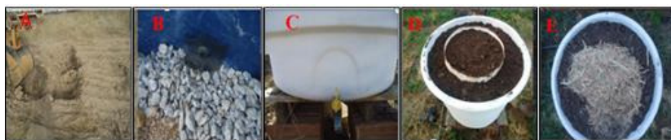
Fig. 3. Soil collection area to fill lysimeters (A), gravel and coarse sand layer (B), drain outlet (C), lysimeter filling with the cylinder in the center (D) and cover with crushed corn husk (E).
