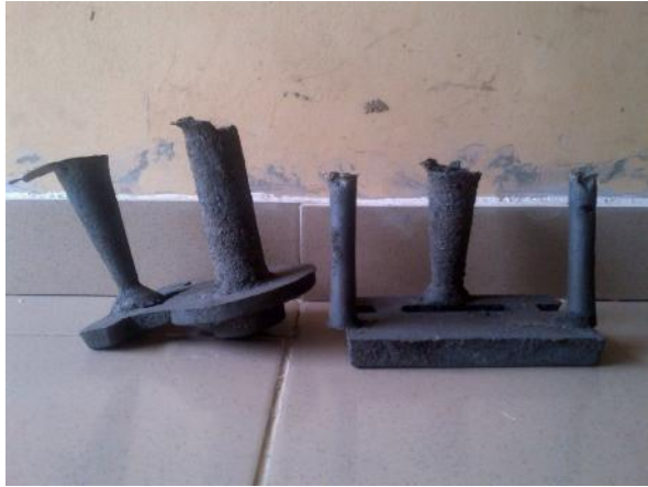
Figure 11: As-cast components in grey cast iron components
