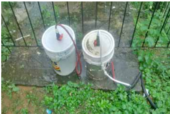
Figure 1: The fabricated digester
