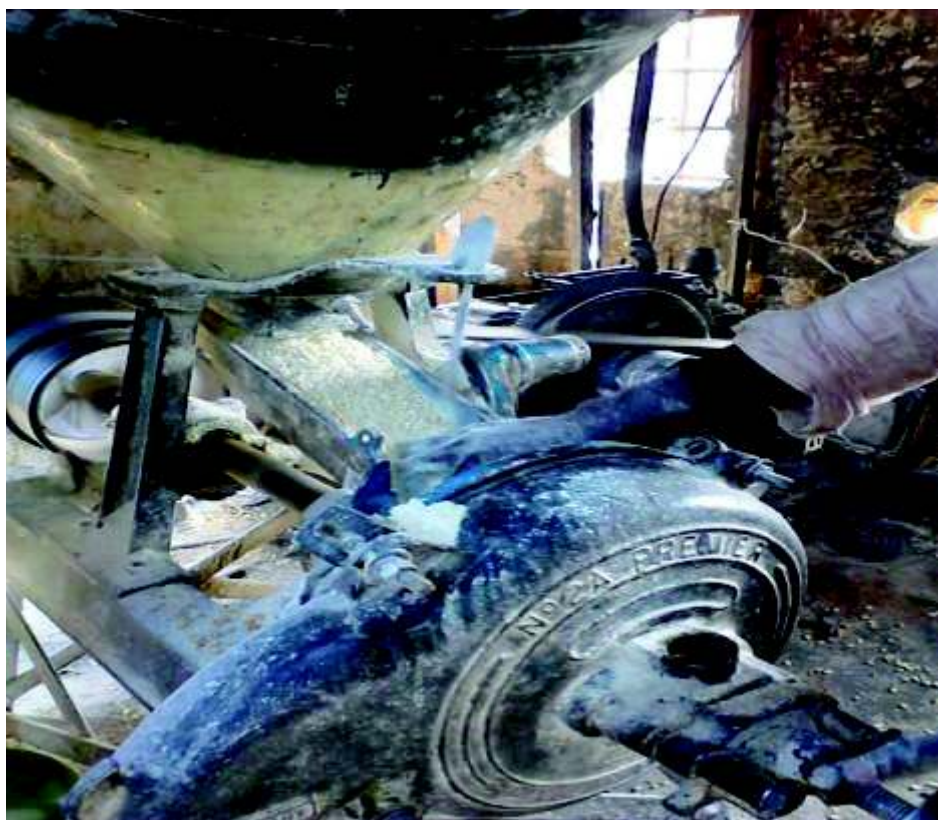
Plate 2.2 : photograph showing “Premier” 127 grinding mill.
