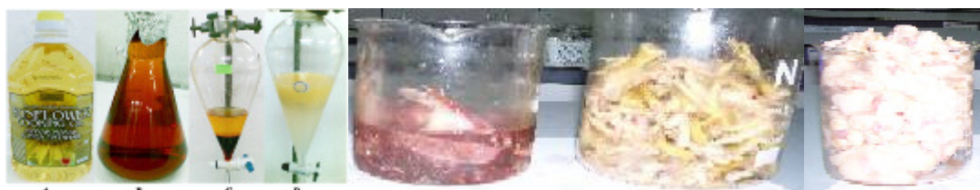
Figure. 1. A) Straight sunflower oil, B) Filtered waste sunflower cooking oil, C) Phase separation, upper is biodiesel and D) Formation of emulsion
