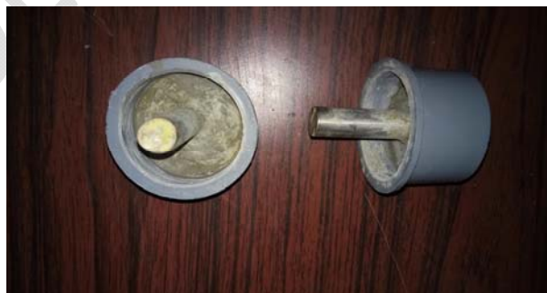
Fig. 4. Electrode using in ohmic heating model for parboiling of paddy.
