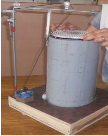
Plate a- Placing the SS plate on the sample
