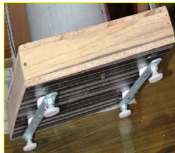
Plate 3- Rectangular wooden box with four adjustable screws
