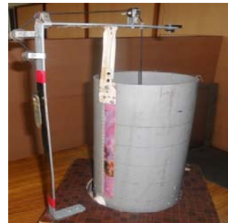
Plate 4- Vertical supporter with four pullies
