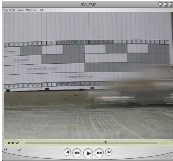
Figure 3. a-b: Two frames of the camera imaging of dynamic speed trap tests
