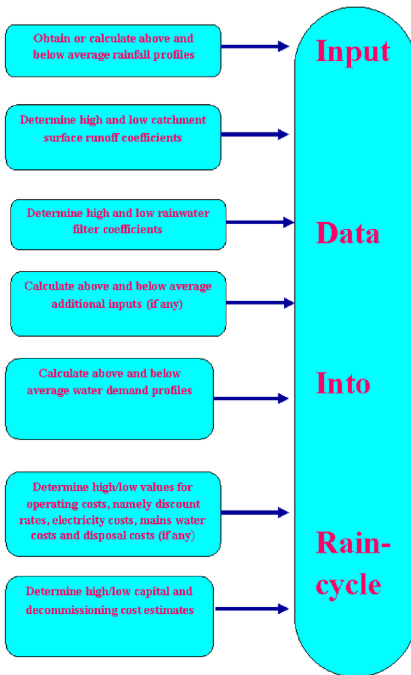
Fig. 6. Assembling data required for detailed analysis
