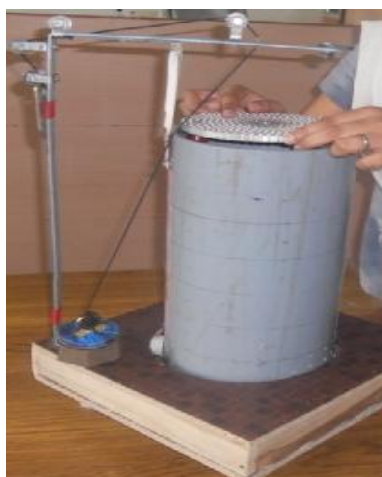
Plate a- Placing the SS plate on the sample
