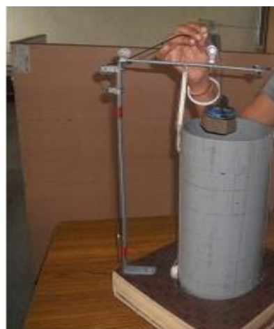
Plate b- Placing the load on the SS plate
