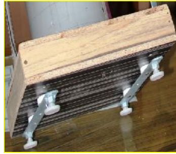
Plate 3- Rectangular wooden box with four adjustable screws
