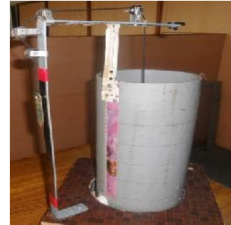
Plate 4- Vertical supporter with four pullies
