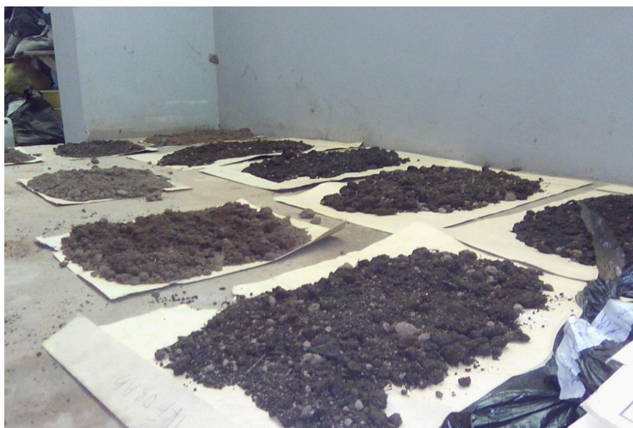
115 Plate 1: Air Drying of Sections of Collected Samples of Soil Mixed and Unmixed with 116 Fuel of Generators Prior to Analysis in the Laboratory 117
