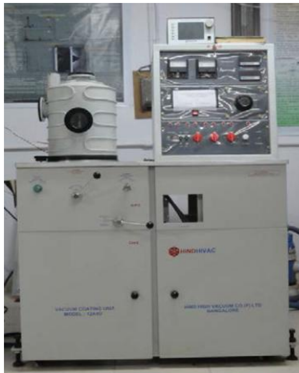
Figure 2: A model-12A4D Vacuum Coating machine employed for Ni-coating of SiC particles
