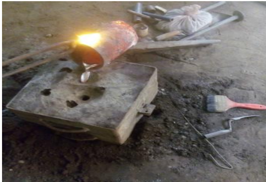
Figure 3: Cast preparation by pouring the Al/SiC slurry from the crucible into the mould
