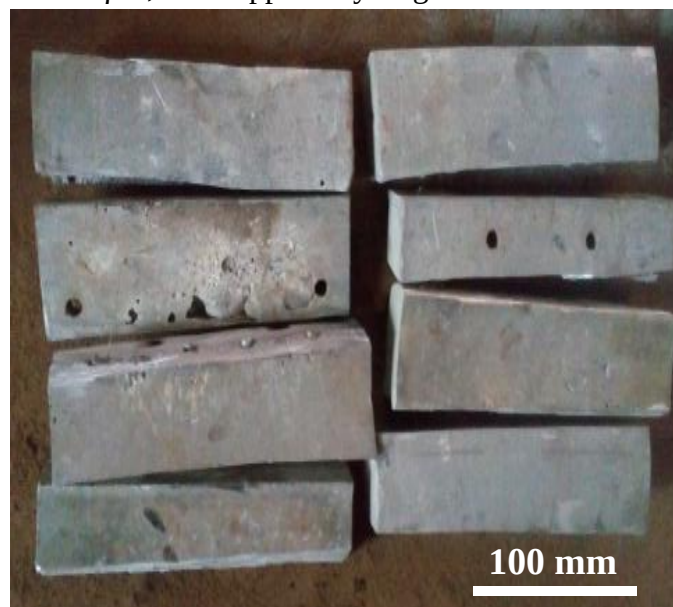
Figure 1: Aluminum Al-4043 alloy lumps used in the study
