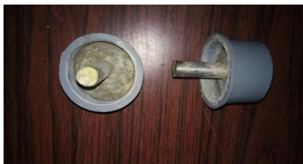
Fig. 4. Electrode using in ohmic heating model for parboiling of paddy.
