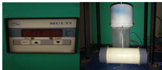
Fig. 3. Temperature controller and sensor for ohmic heating system.
