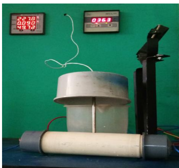
234 235 Fig. 6. Ohmic heating setup for parboiling of paddy.
