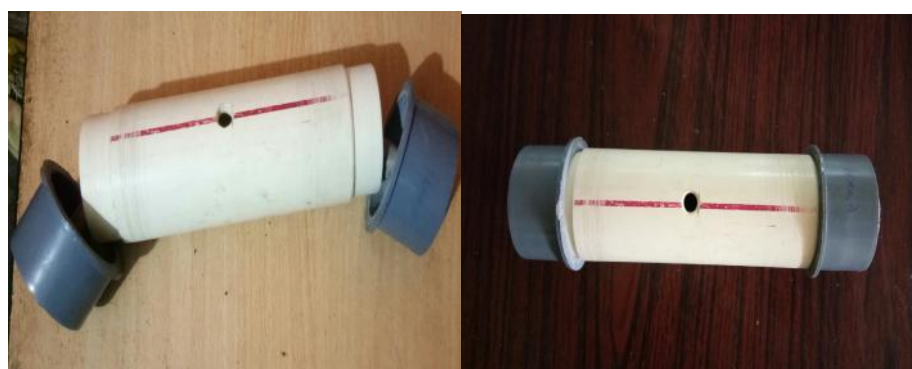
Fig. 2. Ohmic heating chamber for paddy.
