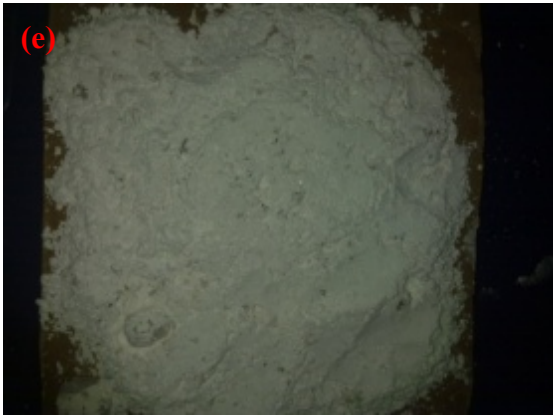
Fig. 1: (a) Raw palm kernel shell (PKS), (b) Grounded palm kernel shell (PKS), (c) Phenolic resin, (d) Steel slag, (e) Grounded iron waste
