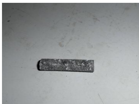
Fig.11. Pitting corrosion of sample in acidic medium
