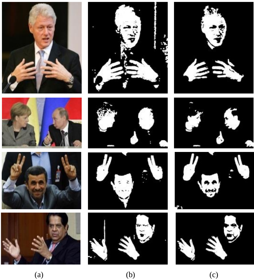
Figure 7: Skin segmentation results: (a) Original images, (b) Segmentation without V information, and (c) Segmentation with V information.
