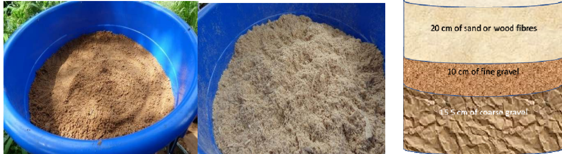
Fig. 1. Top view of sand filter and wood fibres filter before feeding
