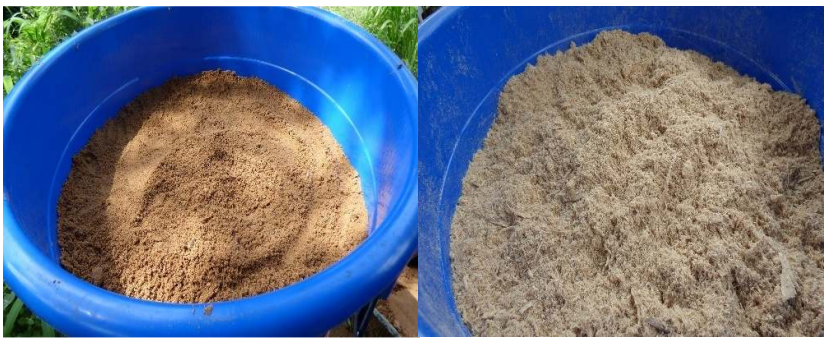
Fig. 1. Top view of sand filter and wood fibres filter before feeding
