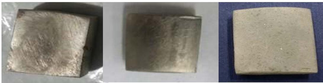
Fig 6: Electroless Ni-P with nano Al 2 O 3 Fig 7: Electroless Ni-P coating Fig 8: Electroless Ni-P coating with nano CuO
