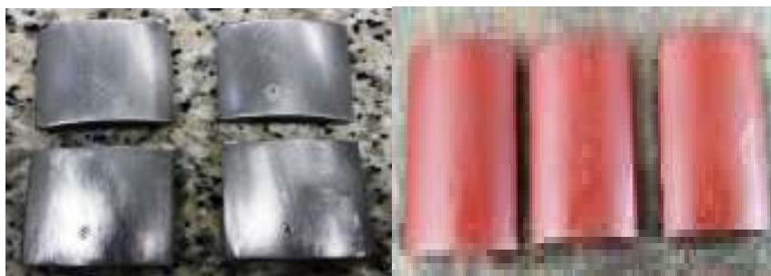
Figure 1: Samples after Mechanical / Chemical polishing and after applying primer
