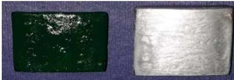
Figure 4: Samples after organic and aluminum paint with nano additive
