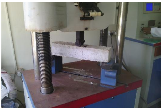
Fig. 3. Specimens undergoing flexural test
