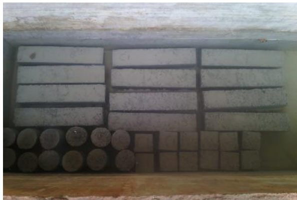
Fig. 2. Samples of specimens water cured
