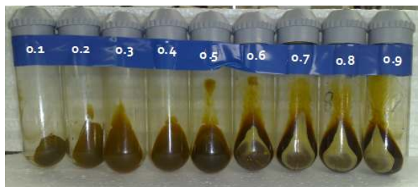
Figure 2: Sludge obtained by centrifugation of different [\text{Fe}^{2+}]/[\text{H}_2\text{O}_2] relationship
