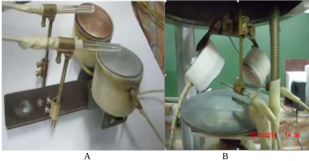
Fig.(4) (a) Langmuir probe with its stand and (b) Langmuir probe setup in system.
