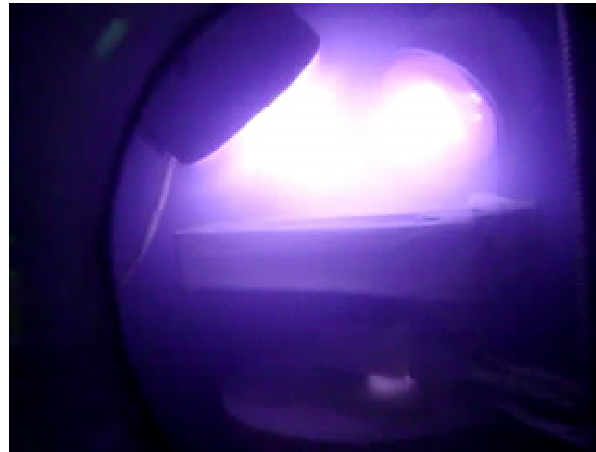
Fig.8 The glow discharge plasma for Cu-Al target
